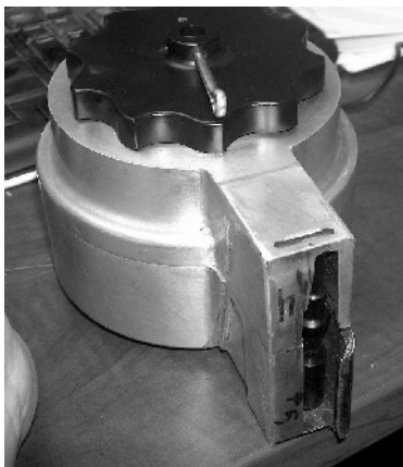
Empty Drum Magazine (cotter pin to show rotation)
