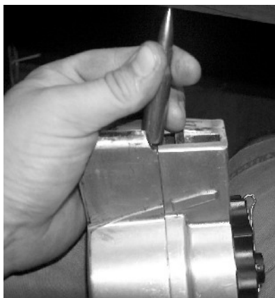
Using the next cartridge to force down the stack as turning hand wheel
